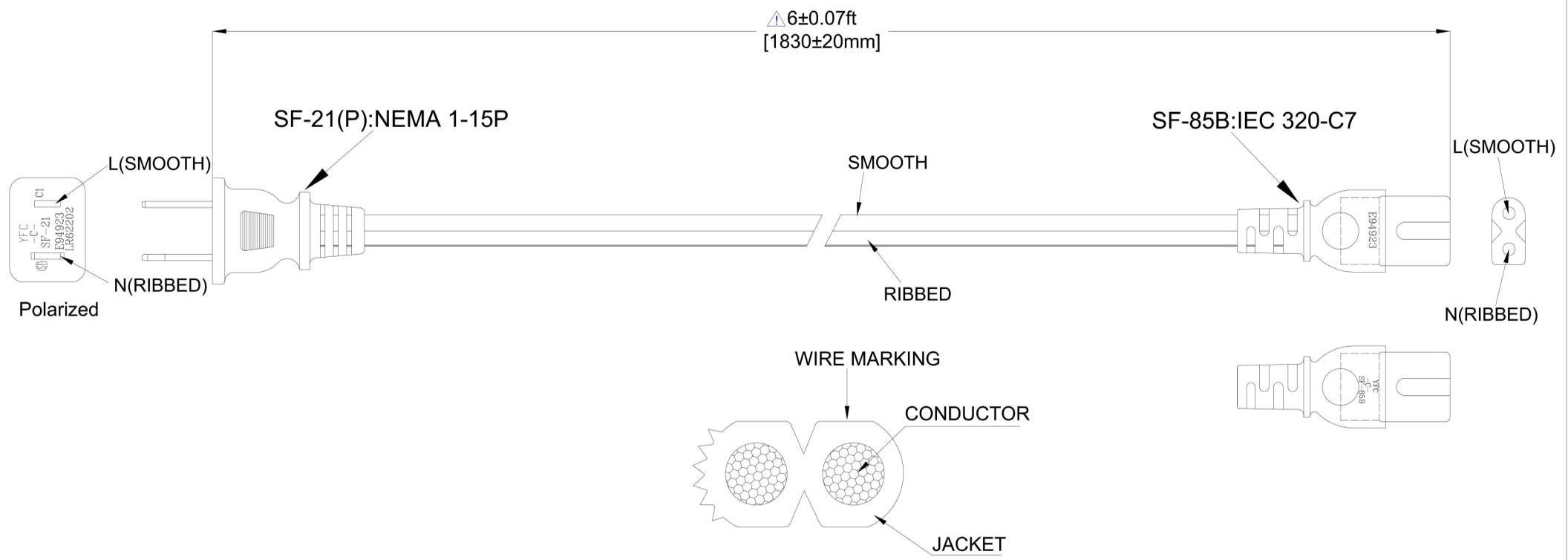
**WIRE MARKING:** (UL) E135710-F3 SPT-2 2X18AWG 60°C 300V VW-1 CSA LL95737
